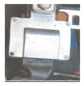
Pin Connector's - On floor retractors are used for attaching the lap belts to the two rear floor retractors. On a regular (manual) lap/shoulder belt assembly, a pin connector button is also on the male portion of lap belt to connect the shoulder belt to the lap belt. The
