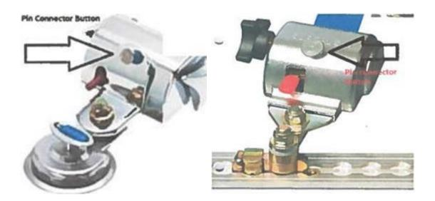
RED RELEASE LEVER - is used to disconnect the J-Hook from the attachment point on the wheelchair. Check to ensure the red release lever is functioning. Pull out and hold the floor retractor webbing. Next, press red release lever - it should release and retract the webbing back into metal housing.
